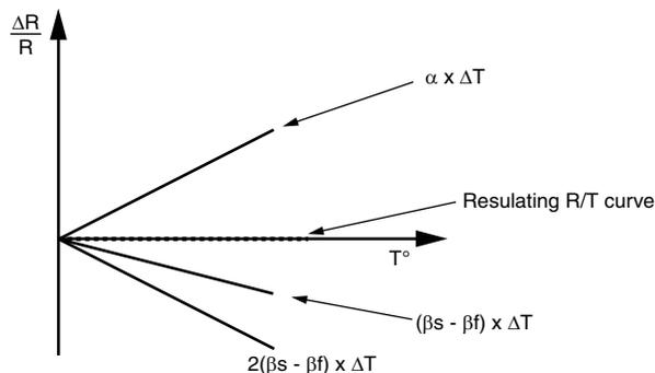
Fig. 5 - Resistance Change of the Free Foil with Change of Temperature.  $\alpha\Delta T$  is Counteracted, after Bonding, by the Strain Gage Effect,  $2(\beta_s - \beta_f)\Delta T$
