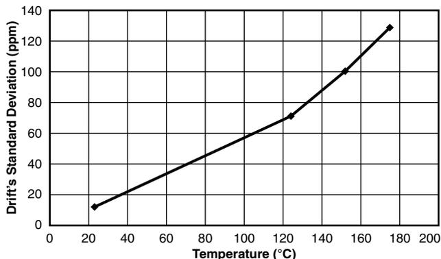
Fig. 1 - 10 000 h Drift's Standard Deviation as Function of Foil's Temperature
