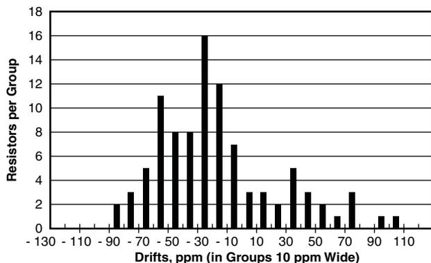
Fig. 3 - Histogram of Drifts for Endurance Testing of 96 Resistors, 10 kΩ, VFR Style S102C
