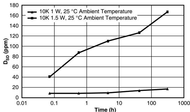
Fig. 4 - Standard Deviation of Drift over 13 Days for 10K VFR S102C Style Resistors at 25 °C at 1 W and 1.5 W. Nominal Power for this Style is 0.6 W at 70 °C.
