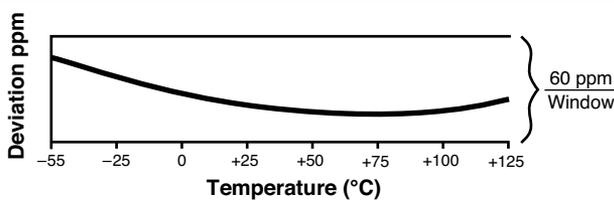
**Figure 3 – Typical Curves Within the 60 ppm Window, VHP10x TCR for Mil Range**
