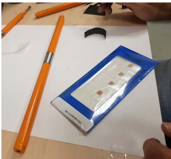
Fig 6: Micro-Measurements® strain gauges
