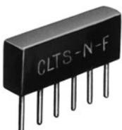
When used in a test program that includes strain gage instrumentation, it is convenient to modify the CLTS output with a simple, passive resistance network as described for LST networks and TG Sensors.
