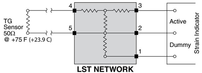
To optimize performance, separate network designs are available for select temperature ranges covering cryogenic to +500°F. The environmental temperature range for LST networks is -65° to +250°F (-55° to +125°C). Standard strain gage instrumentation, such as the Micro-Measurements Model P3, is ideal for use with these sensors, eliminating the need to purchase separate readout devices.
