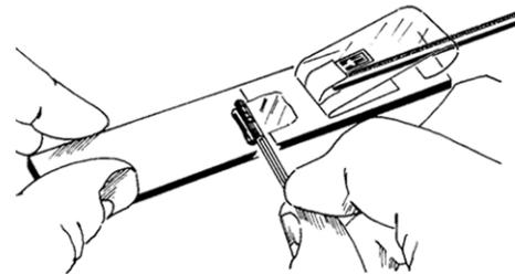
After the adhesive has cured, remove the transfer tape by pulling it back directly over itself, peeling it slowly and steadily off the surface. An application of RSK-1 Rosin Solvent will quickly soften the mastic and ease tape removal. Then, gently lift the cable and jumper wires and remove the Teflon film.
