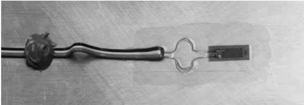
After the cable has been properly anchored, the remainder of the bundled cable can be unsecured and routed to the strain gage instrumentation. If a cable extension is added, remember that it should be attached by soldering. Alligator clips, twist caps, and most other mechanical connections should be avoided when making electrical connections within strain gage circuits.
