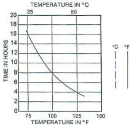
**Note:** Potted connectors or coatings of M-Coat JA that exceed 3/8 in [10 mm] in thickness should be air dried for 2 hours at room temperature prior to starting an elevated-temperature cure.
