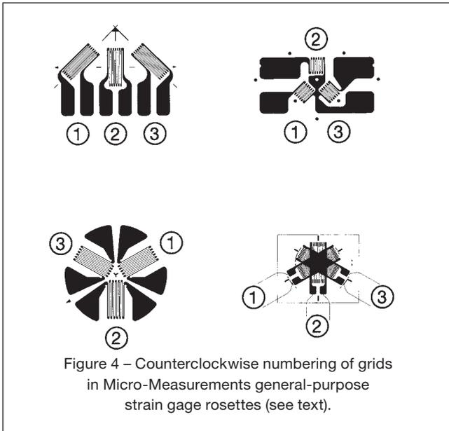
Micro-Measurements stacked rosettes are not numbered, as a matter of manufacturing economics. The user should number the gages in stacked rosettes according to the rules given here and illustrated in Figures 2 and 4.
