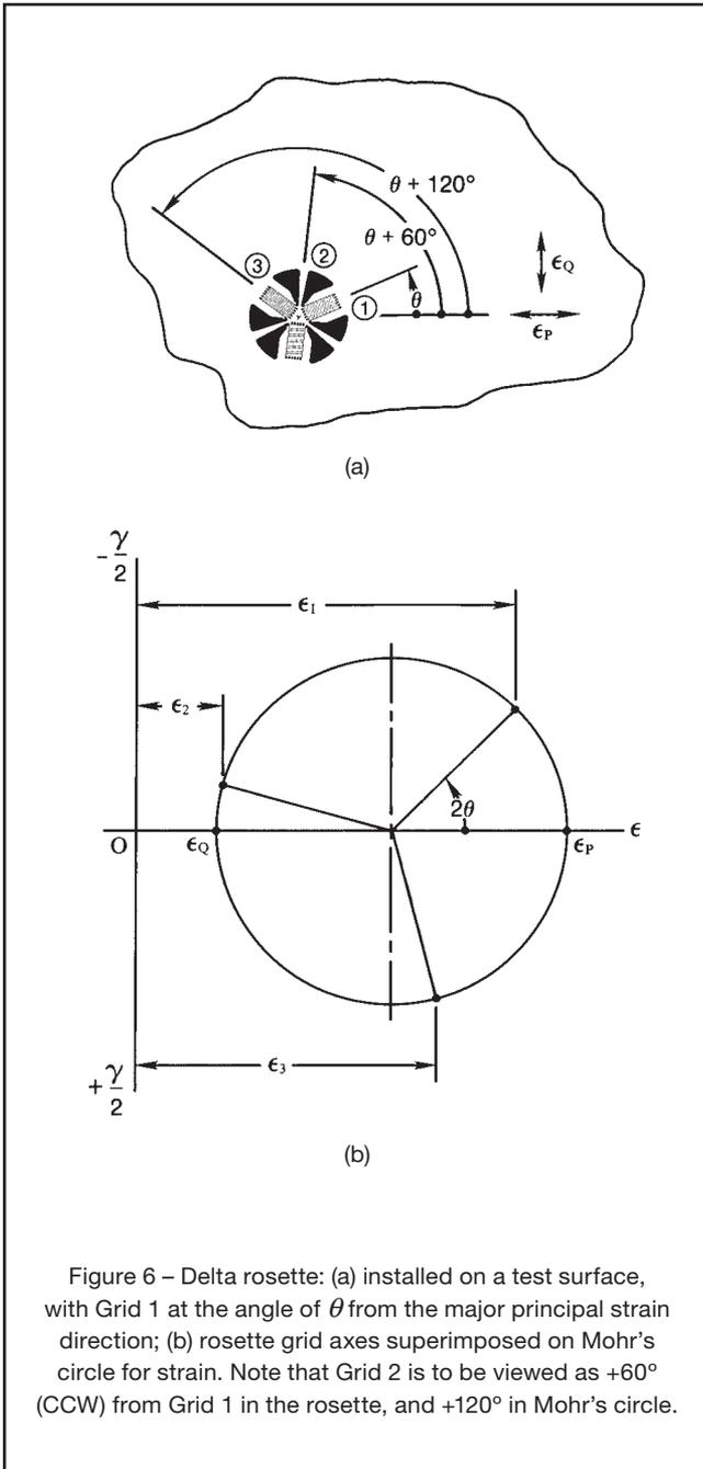
Figure 6 – Delta rosette: (a) installed on a test surface, with Grid 1 at the angle of  $\theta$  from the major principal strain direction; (b) rosette grid axes superimposed on Mohr's circle for strain. Note that Grid 2 is to be viewed as  $+60^\circ$  (CCW) from Grid 1 in the rosette, and  $+120^\circ$  in Mohr's circle.
