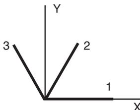
The foregoing assumes in each case that the gage elements in the rosette are numbered counterclockwise as indicated. When the calculated  $\gamma_{XY}$  is positive in sign, the initial right angle at the origin of the X-Y coordinate system is decreased by the amount of the shear strain.
