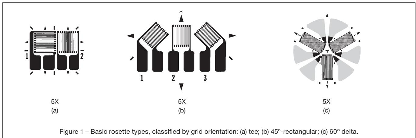
Figure 1 – Basic rosette types, classified by grid orientation: (a) tee; (b) 45°-rectangular; (c) 60° delta.
