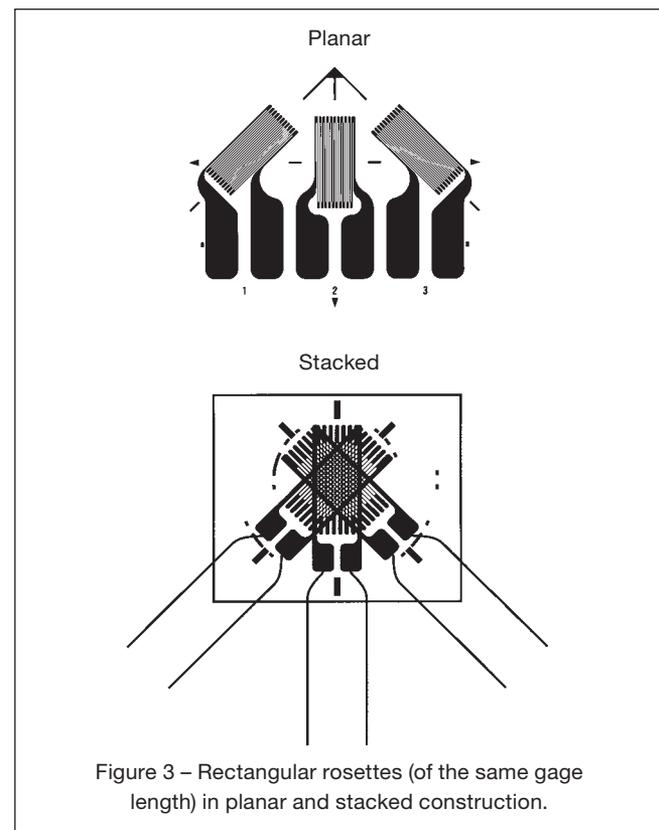
Figure 3 – Rectangular rosettes (of the same gage length) in planar and stacked construction.
