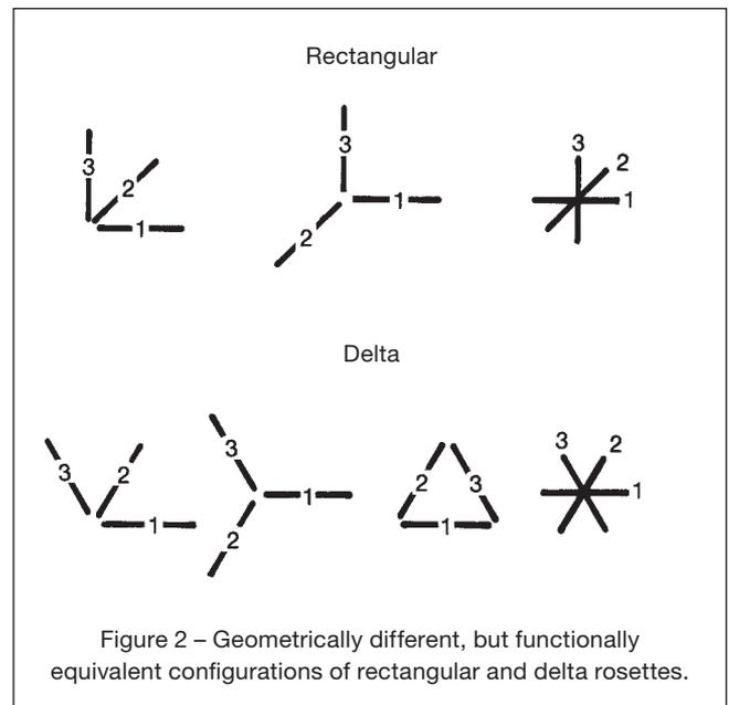
Figure 2 – Geometrically different, but functionally equivalent configurations of rectangular and delta rosettes.
