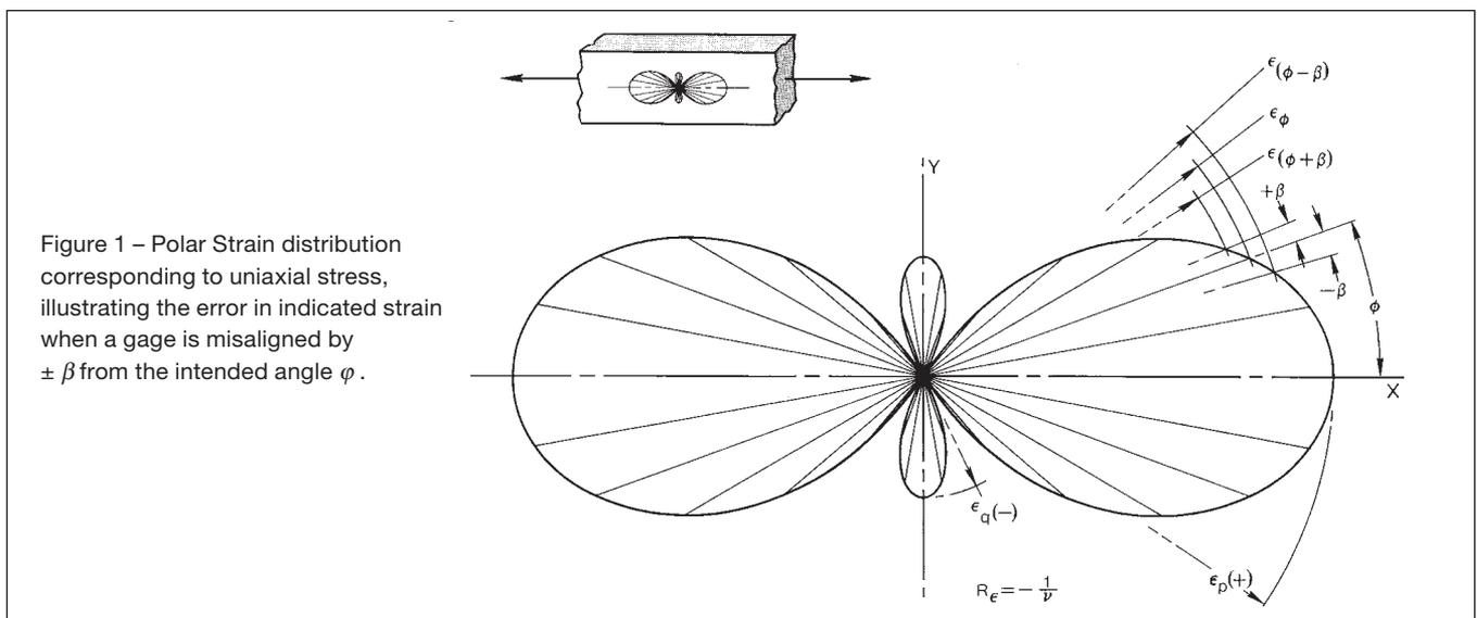
Figure 1 – Polar Strain distribution corresponding to uniaxial stress, illustrating the error in indicated strain when a gage is misaligned by  $\pm \beta$  from the intended angle  $\phi$ .
