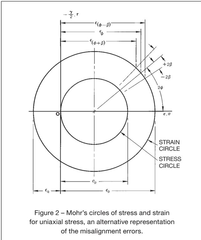
Figure 2 – Mohr's circles of stress and strain for uniaxial stress, an alternative representation of the misalignment errors.
