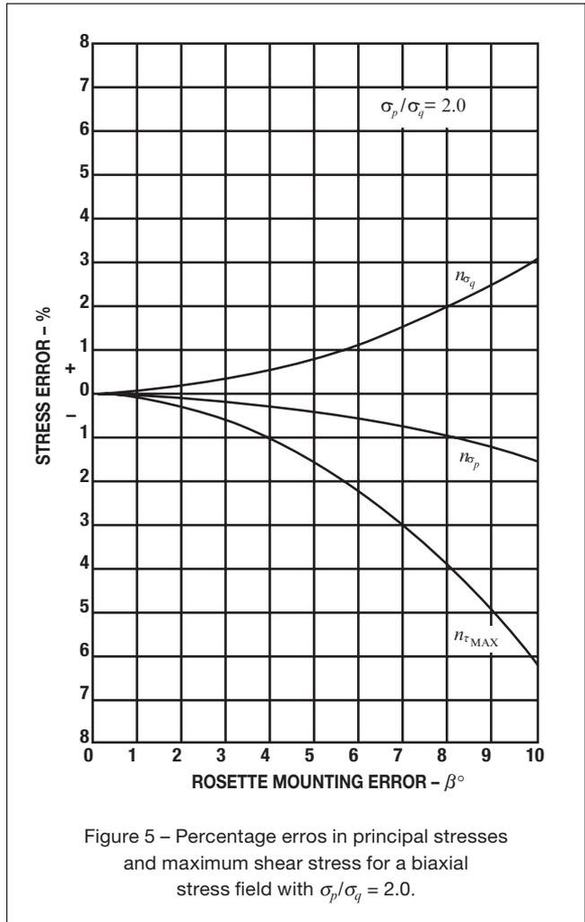
Figure 5 - Percentage errors in principal stresses and maximum shear stress for a biaxial stress field with  $\sigma_p/\sigma_q = 2.0$ .
