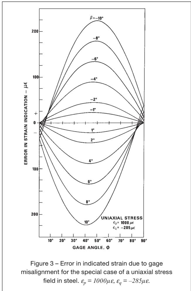
Figure 3 – Error in indicated strain due to gage misalignment for the special case of a uniaxial stress field in steel.  $\epsilon_p = 1000 \mu\epsilon, \epsilon_q = -285 \mu\epsilon$ .
