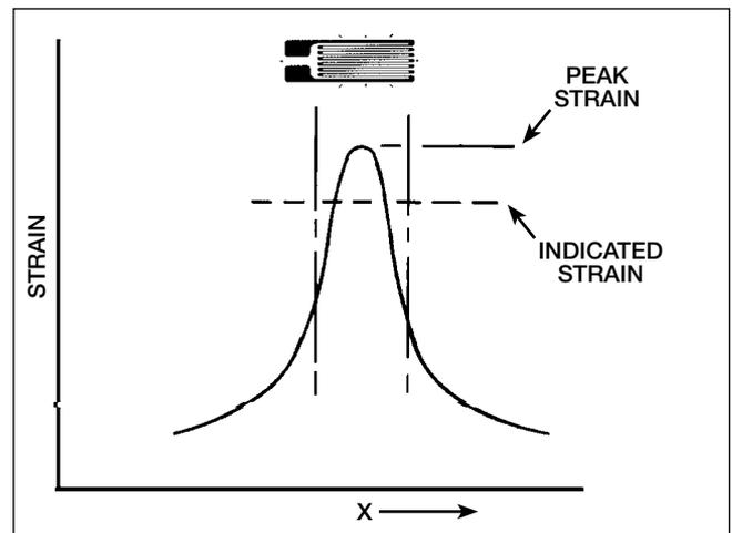
strain over the area covered by the grid. Since the average of any nonuniform strain distribution is always less than the maximum, a strain gage which is noticeably larger than the maximum strain region will indicate a strain magnitude that is too low. The sketch above illustrates a representative strain distribution in the vicinity of a stress concentration, and demonstrates the error in strain indicated by a gage which is too long with respect to the zone of peak strain.
