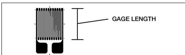
experimental stress analysis and transducer applications, Micro-Measurements offers gage lengths ranging from 0.008 in (0.2 mm) to 4 in (100 mm).
